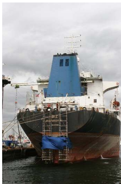
RIGHT: Towed into Cape Town some time ago with a vegetable oil cargo, Biz is undergoing rudder replacement.
