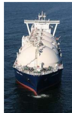
RIGHT: Grand Aniva , an example of the Kvaerner-Moss Containment System
