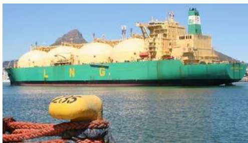
TOP: LNG Cross River , another with the Kvaerner-Moss system that makes these gassers so conspicuous.
