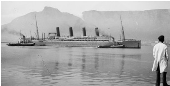
TOP: Arundel Castle , built with four funnels and modified during a refit shortly before World War 2 from which she emerged with a clipper bow, more powerful oil-fired engines and two funnels. She was withdrawn in December 1958 after 37 years' service.
